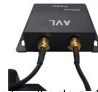
Connect the GSM Antenna to the unit.
