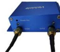
Find a suitable place inside the car for installing the unit. Wiring connections must be firm and reliable and the joints should be wrapped with insulating tape tightly. The unused electrical wire should be properly insulated.
